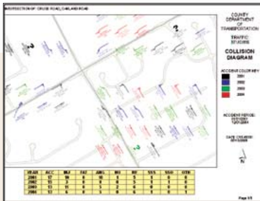
Example of a Midblock Collision Diagram That Includes Aerial Photos and Road Centerlines
